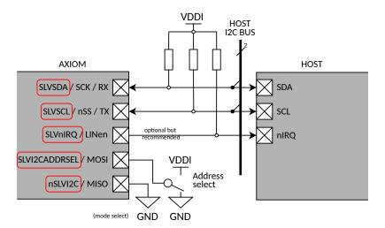
Figure 7.3.2-1: Slave I<sup>2</sup>C Connections
