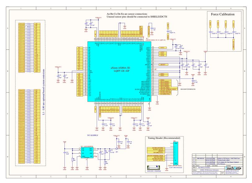
Figure 5-1: Reference Schematic (LQFP128)
