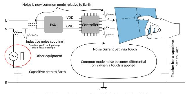
Figure 6.7-1: Example Common Mode Noise From "Other" Equipment
