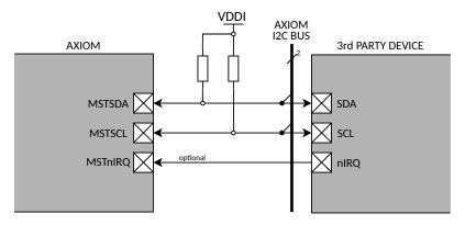
Figure 8-1: Master I<sup>2</sup>C Connections to 3<sup>rd</sup> Party Device(s)
