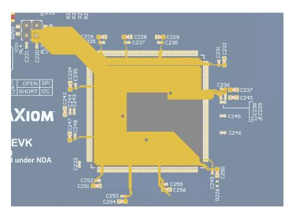
Figure A.1.1-1: C-shaped power routing, balanced amongst all VDDA pins. Figure shows an AX198A, same advice can be applied to this device.
