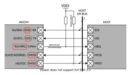
Figure 7.4.2-1: Slave SPI Connections
