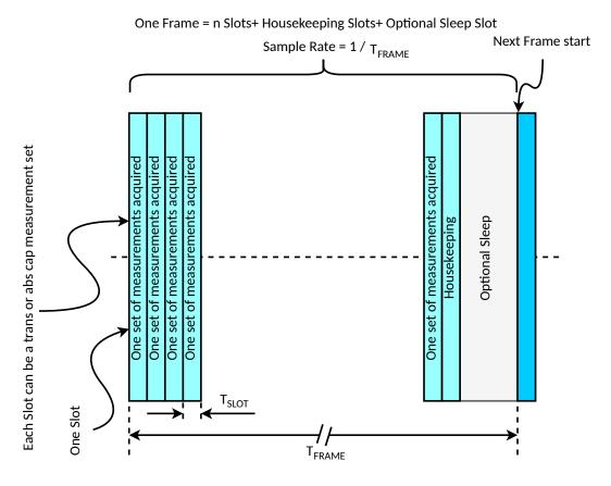
Figure 6.1-1: Acquisition Engine Frame Structure
