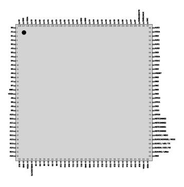
Figure 3.1.1-1: LQFP128 Device Pinout (top view)
