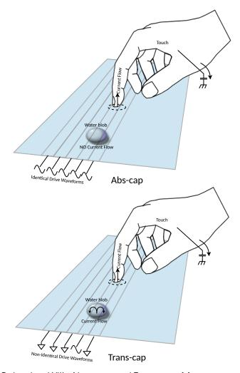
Figure 6.8-1: Different Behaviors With Abs-cap and Trans-cap Measurements With Water and Touch
