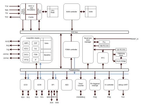
Figure 6.1-2: Simplified System Architecture
