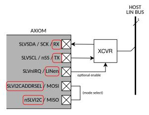
Figure 7.5.1-1: Slave LIN Connections
